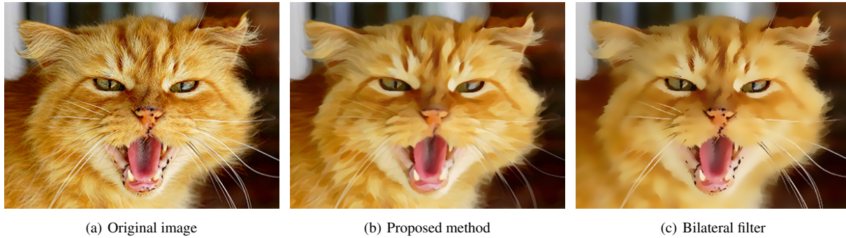
Figure 10: In contrast to the bilateral filter our approach avoids overblurring in low-contrast regions.
